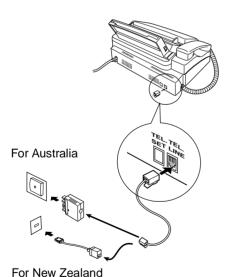
Be sure to insert the telephone line cord into the **TEL. LINE** socket. Do not insert it into the **TEL. SET** socket.
